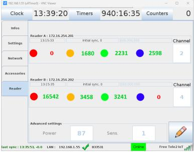
If there is still **0**, the cable or the antenna may have a fault.
