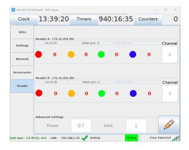
In the device, the notion of channel is present in the section Settings then Reader. If you click on the pencil, you will be able to modify channels.
